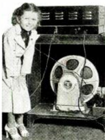
The 20-tube Masterpiece V, showing the giant 18" speaker. Betty Titus stands less than 4 feet tall.
