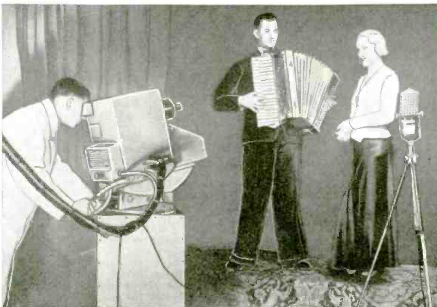
A view in the Philips television studio, showing pickup of image for 405 line scanning; the mike for picking up the sound appears at the right of the picture.
